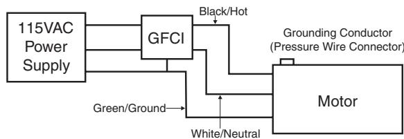
**ELECTRICAL REQUIREMENTS** Every Jentle Ped foot spa is supplied with a 1 bhp, 110 Volt pump that draws 5.5 amps. It comes with a 29" grounded plug to be plugged into a standard grounded receptacle. You will need a 15 amp line with a GFCI outlet. The pump is activated by a deck-mounted on/off control.
